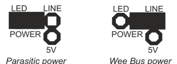
Fig.3 Jumper POWER - Power source configuration
